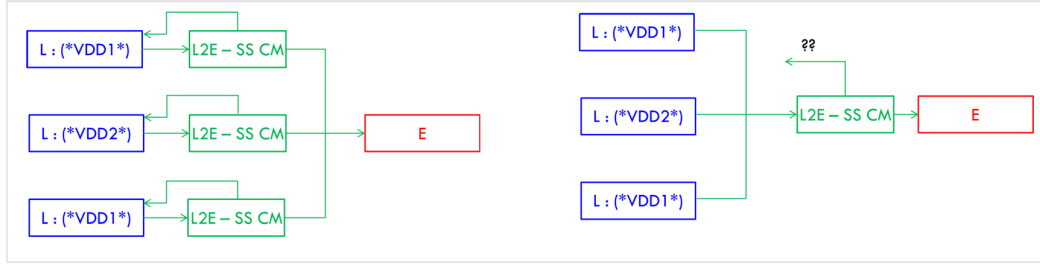
Figure 7. Fanout signal causing sub-optimal SS CM insertion
